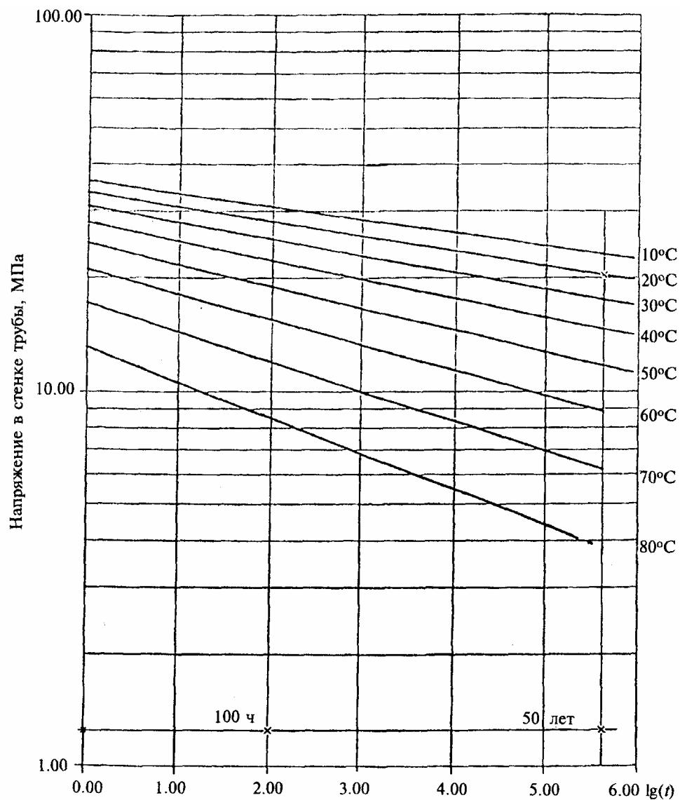
$$\lg(t) = -121,699 - (25985/T) \lg(\sigma) + 47143,18/T + 63,03511 \lg(\sigma),$$
