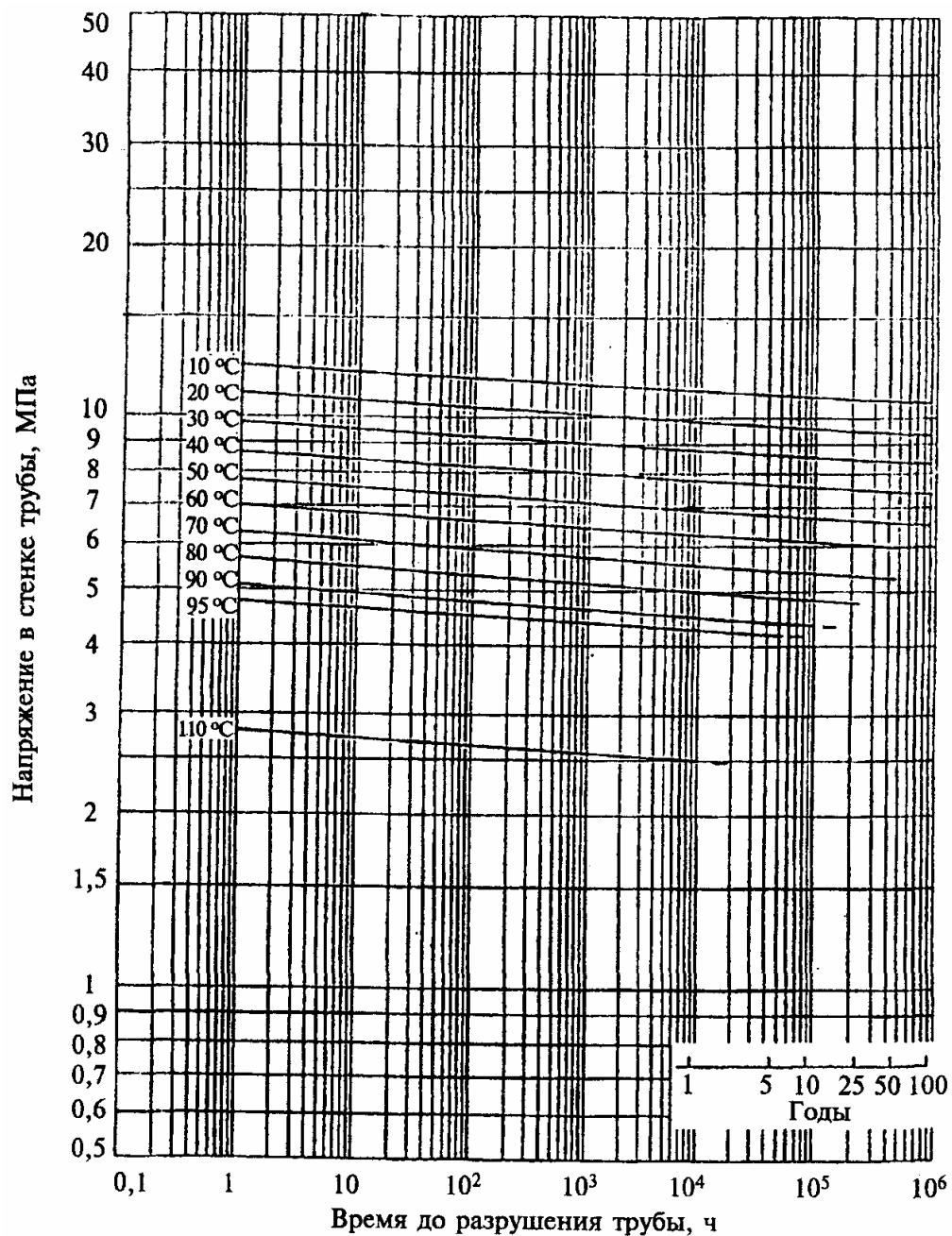
$$\lg(t) = -105,8618 - (18506,15/T) \lg(\sigma) + 57895,49/T - 24,7997 \lg(\sigma),$$
